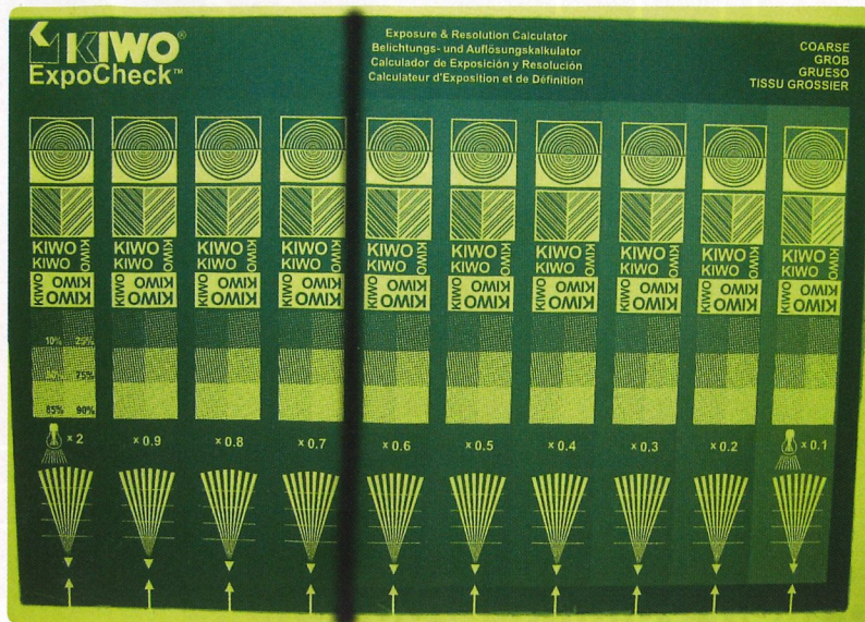
Figure 2: This exposure test shows a black line at the point where there is no rectangular filter covering the emulsion. All exposure steps left of the black line show no color variation between the facing arrows along the bottom of the stencil, while exposure steps right of the line do.
