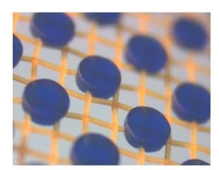
**KIWOCOL® POLY-PLUS HWR** produces a <u>Highly <u>Water Resistant</u> stencil designed for use with water-based inks in long run applications. Due to its high mechanical and abrasion resistance, **KIWOCOL® POLY-PLUS HWR** is also ideal for ceramic inks as well as roll to roll printing of wallpaper, rugs, glass and other abrasive substrates. It can be chemically hardened with KIWO'S HARDENER K to create a permanent stencil.</u>
